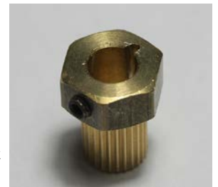
It helps to file a slot a slot where the wire bulges a bit
